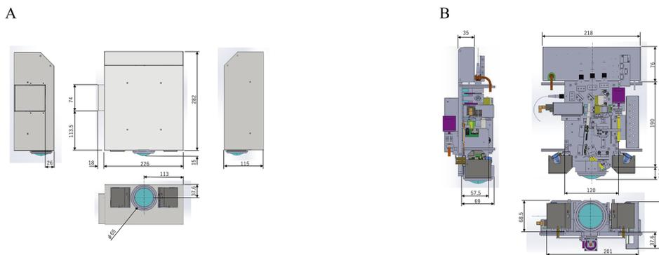
Fig. 1. External and internal dimensions of the semiconductor laser-based SLO system.
