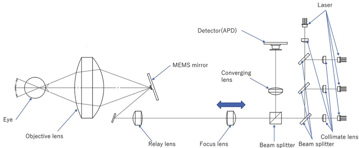
Fig. 2. Schematic and optical design of the SLO system.
